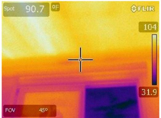
LOCATION: Main floor. EQUIPMENT: Ceiling over sliding glass door. NOTE: Thermal signature corresponding with stains on ceiling appear to be from exhaust vents in ceiling. Inspector thinks stains could be from deteriorating sealant on exterior of building where exhaust vents terminate. Condensation from uninsulated exhaust ducts may also be contributing to stains on ceiling.
