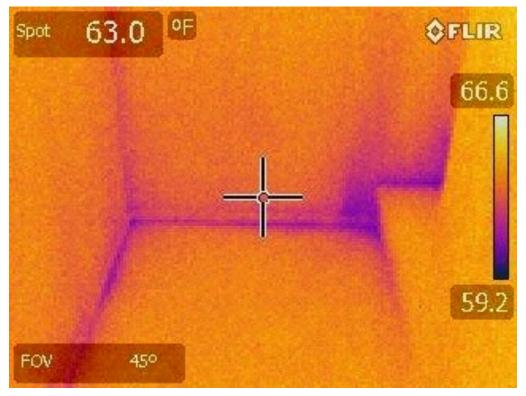
LOCATION: Downstairs at bottom of stairway. EQUIPMENT: Interior wall NOTE: No thermal signature noted that suggested water intrusion around the attachment to the house.
