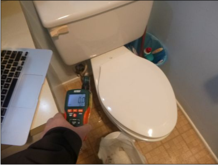
Elevated moisture levels in sub flooring.
